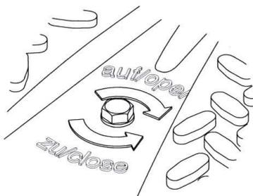
Turning the hexagonal head of the screw on the top of the lid (B) opens and closes the safety latch. The latch locks into a slot or into the inner edge of the inspection chamber. (Point 2.2.1)
