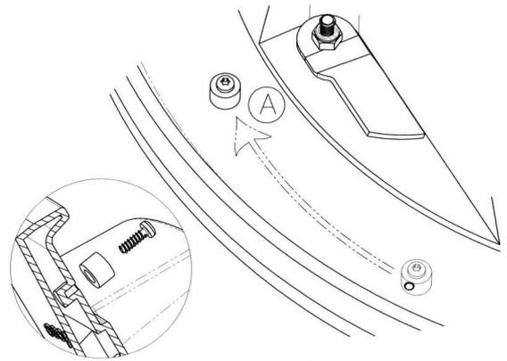
The figure on the right shows the safety latch lock in an inspection chamber in the closed position.
